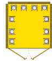
PAN05 - LED10 For 10 gas cylinders W1760 x D1680 x H2400mm Weight: 550 Kg
